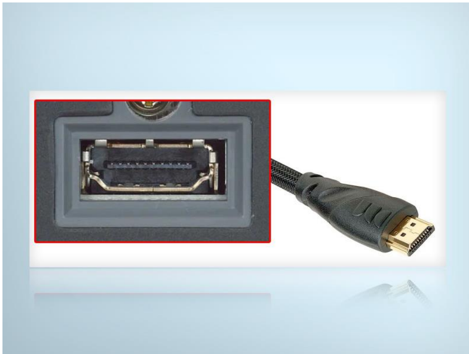
Figure 39: HDMI jack and connector
